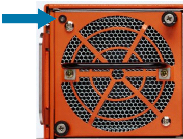
Figure 6 Individual Fan LED Location on GigaVUE-HC3 Rear
